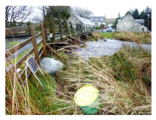
Figure 34 Crosswater of Luce sample point during high flow conditions showing the automatic sampler dislodged and separated from its green and yellow stand.
