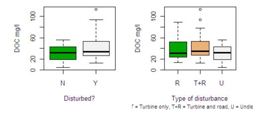
Figure 75. DOC concentrations (mg L<sup>-1</sup>) from Arecleoch spatial survey samples points comparing (a) median values between disturbed (Y) and undisturbed (N) sites and (b) sites subject to disturbance from road building only (R), turbine installation and road building (T+R) and not disturbed by wind farm activities (U)
