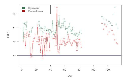
Figure 95. E4/E6 ratios for T33 upstream and T33 downstream samples. samples collected on consecutive days are shown connected by a line. Day  $1 = 3^{rd}$  February 2010. The horizontal line indicates a nominal transition between humic (<5) and fulvic (>5) substances
