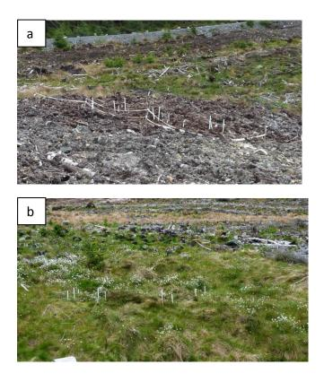
Figure 92. a) Peat store and b) control site at Arecleoch wind farm. Nests of piezometers are visible distributed across the area.
