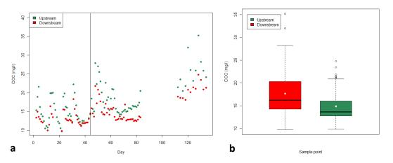
Figure 85. (a) Time series of DOC concentration against day (Day 1 = February 2<sup>nd</sup> 2010) upstream and downstream of turbine base installation T33. The vertical line indicates the date at which work on T33 was completed according to SPR records. (b) Range of DOC concentrations upstream and downstream of turbine base installation T33. White dot represents mean values
