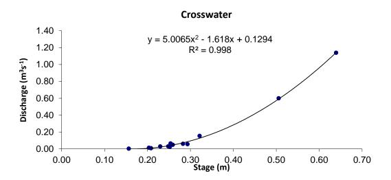
Figure 32. Rating equation for the Crosswater showing the relationship between discharge (m<sup>3</sup>s<sup>-1</sup>) and stage (m) and giving the resulting rating equation
