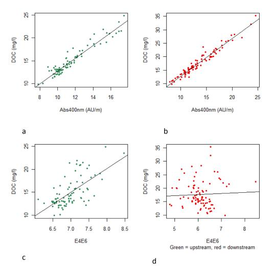
Figure 97. Scatterplots of Absorbance vs DOC concentration for T33 upstream (a) and T33 downstream (b); and E4/E6 ratios vs DOC concentration for T33 upstream (c) and T33 downstream (d). Fitted line for linear regression shown in black.
