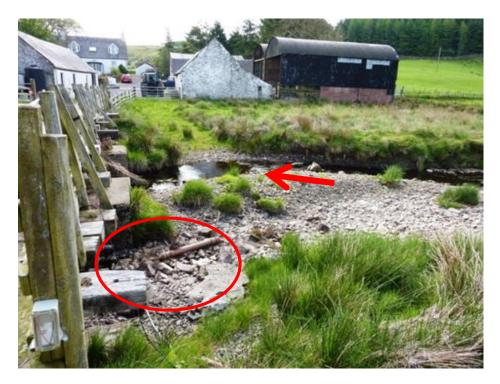
Figure 33. Crosswater of Luce sample point during a prolonged dry period showing exposed instrumentation within the red circle. Water flowed only in a channel on the far side of the gravel bar (indicated by the arrow)
