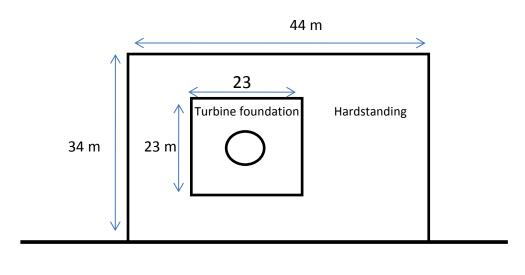
Figure 51. Schematic of the dimensions of a typical turbine base excavation
