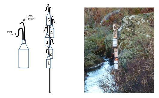
Figure 22. Illustration of a rising stage sampler (left) and image of actual equipment (right) in situ at the Crosswater sample point
