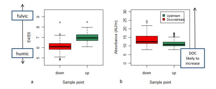
Figure 96. E4/E6 ratios (a) and absorbance at 400 nm for T33 upstream and T33 downstream samples
