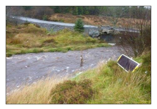
Figure 19. Tig sample point – a cobble/boulder bed stream in the heart of Arecleoch forest. The solar panel used to trickle charge the autosampler battery is visible in the foreground
