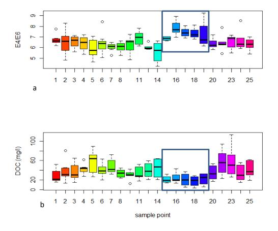
Figure 98. E4/E6 ratios (a) and DOC concentrations (b) for spatial survey samples at Arecleoch. The box in each chart indicates the control sample points 15 - 19
