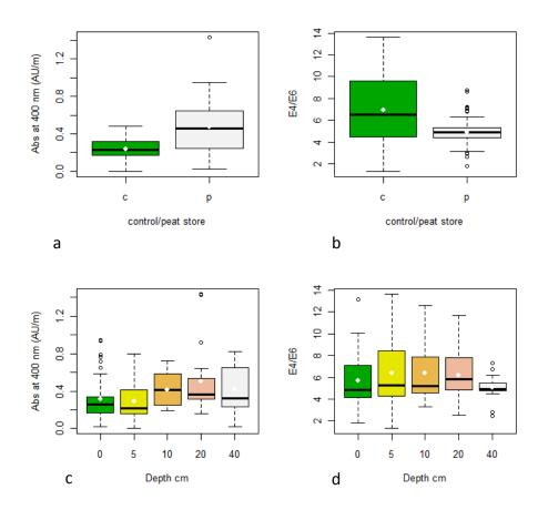
Figure 93. Comparison between pooled data at the peat store and control site for a) absorbance at 400 nm and b) the E4/E6 ratio.
