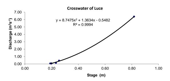
Figure 35. Rating equation for period 1 at the Crosswater of Luce
