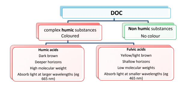
Figure 90. Characterising DOC by dividing into humic and non-humic fractions and further division of the humic fraction into fulvic and humic acids (derived from Bourbonniere (2009)).
