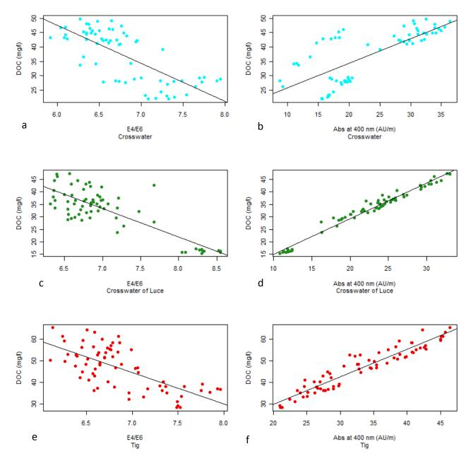
Figure 102. Comparison of E4/E6 ratios with DOC concentration and Absorbance at 400 nm with DOC concentration at the Crosswater, Crosswater of Luce and Tig sample points at Arecleoch.
