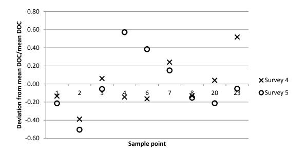
Figure 78. Deviation from mean DOC concentrations as a proportion of mean values for spatial surveys four (Aug 2009) and five (Nov 2009) showing only sample points where samples were obtained on both surveys
