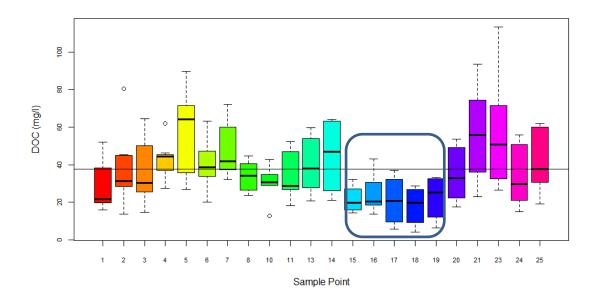
Figure 74. Range of DOC concentrations at the 22 spatial survey sample points. Sample points 15 – 19, within the box, were used as controls.
