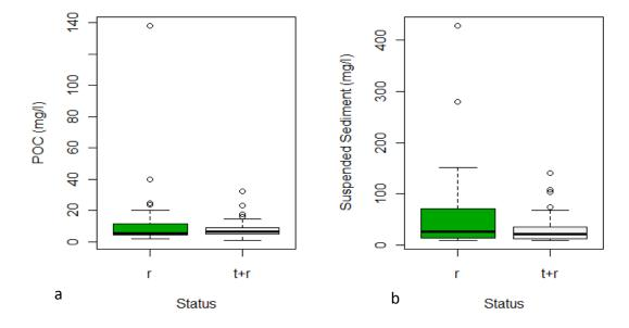
Figure 87. POC (a) and suspended sediment (b) concentrations of pooled data for Arecleoch samples points exposed to disturbance from road building only (r) and turbine installation and road building (t+r)
