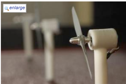
In wind tunnel experiments at Johns Hopkins, air currents pass through a series of small model wind turbines mounted atop posts, mimicking an array of full-size wind turbines. (Credit: Will Kirk/JHU)
